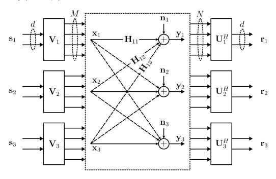
Figure 2.1.: Used MIMO interference channel model
