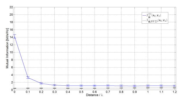
Figure 4.10.: MI of IA as a function of receiver movement, desired transmitter 2, averaged over  $N_M=1000$  measurements with 95% confidence intervals of the mean
