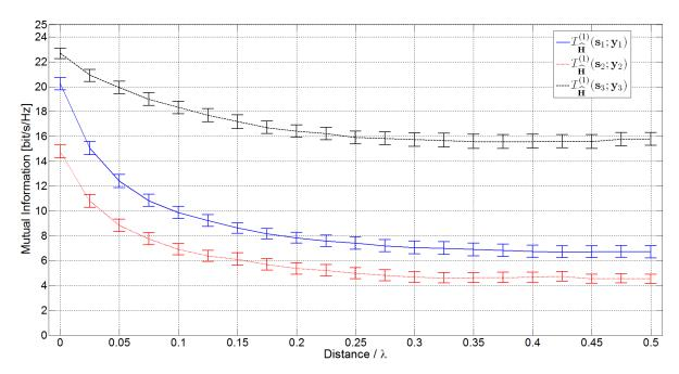
Figure 4.15.: MI of IA as a function of receiver movement over half a wavelength, no receive filters, averaged over  $N_M = 1000$  measurements with 95% confidence intervals of the mean
