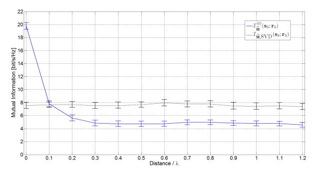
Figure 4.11.: MI of IA as a function of receiver movement, desired transmitter 3, averaged over  $N_M = 1000$  measurements with 95% confidence intervals of the mean
