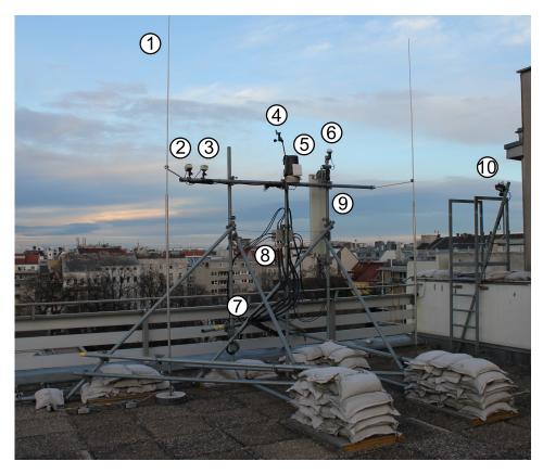
$\begin{array}{c} \textbf{Figure 3.5.:} \text{ Antenna setup of Tx2: 1 lightning arrester, 2 rain sensor, 3 fog sensor, 4 wind speed sensor, 5 precipitation amount sensor, 6 GPS,7 webcam (not visible) , 8 antenna switch, 9 antenna, 10 lamp \\ \end{array}$
