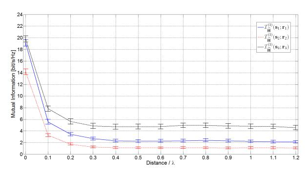
Figure 4.12.: MI of IA as a function of receiver movement, comparison, averaged over  $N_M=1000$  measurements with 95% confidence intervals of the mean
