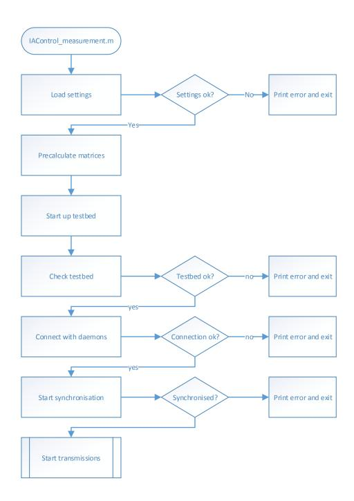
Figure 3.9.: Initialization in the Matlab measurement script at the receiver
