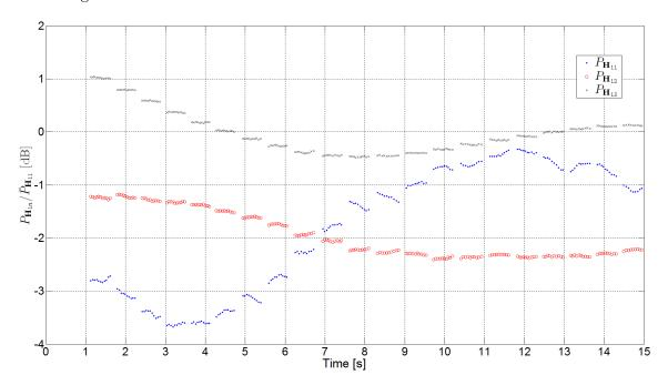
**Figure 4.4.:** Typical measurement of the received power from each transmitter over time, normalized to the average received power from Tx1
