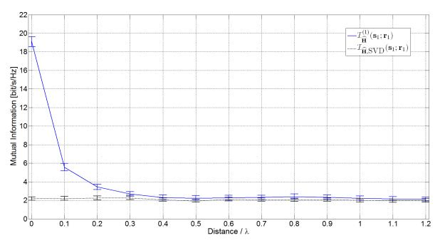
Figure 4.9.: MI of IA as a function of receiver movement, desired transmitter 1, averaged over  $N_M = 1000$  measurements with 95% confidence intervals of the mean
