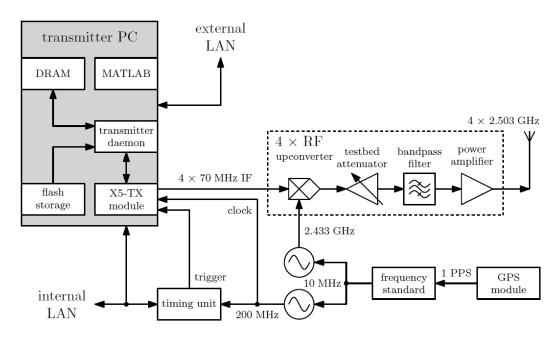
Figure 3.3.: Blockdiagram of the transmitter chain [18, pg. 2, figure 2.1]
