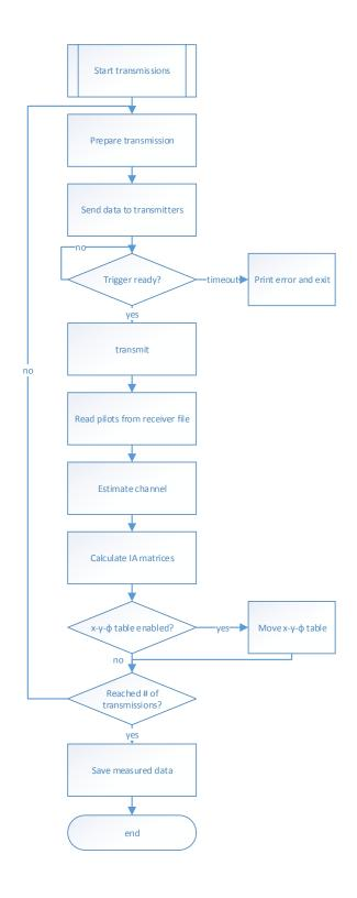
Figure 3.10.: Program flow of the measurement script while transmitting
