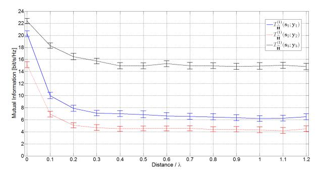
Figure 4.13.: MI of IA as a function of receiver movement, no receive filters, comparison, averaged over  $N_M = 1000$  measurements with 95% confidence intervals of the mean
