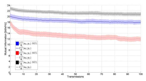
Figure 4.2.: MI with channel changing over time, no receive filters applied, averaged over  $N_M = 50$  measurements with 95% confidence intervals of the mean
