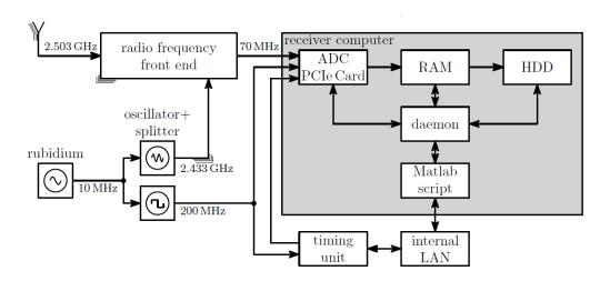
Figure 3.7.: Block diagram of receiver chain [22, pg. 2, figure 1.1]
