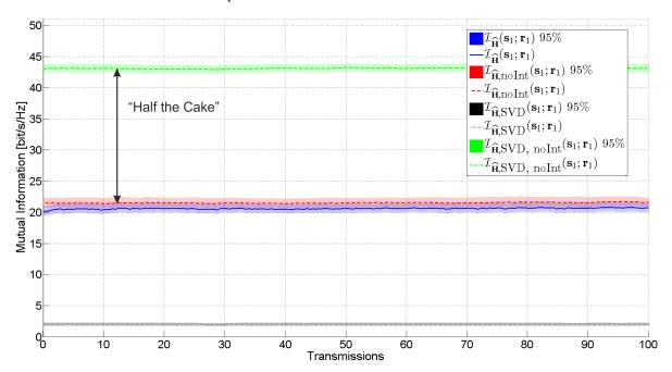
Figure 4.5.: IA, link 1, compared to SVD and IA without interferers, averaged over  $N_M = 50$  measurements with 95% confidence intervals of the mean
