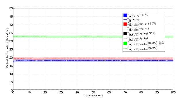
Figure 4.6.: IA, link 2, compared to SVD and IA without interferers, averaged over  $N_M = 50$  measurements with 95% confidence intervals of the mean
