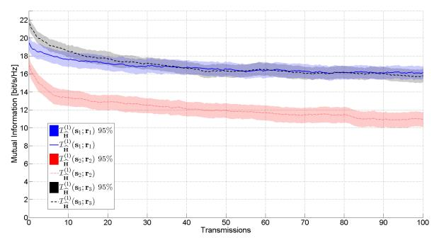
Figure 4.1.: MI with channel changing over time, averaged over  $N_M = 50$  measurements with 95% confidence intervals of the mean
