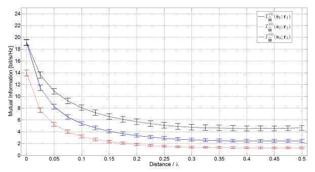
Figure 4.14.: MI of IA as a function of receiver movement over half a wavelength, averaged over  $N_M = 1000$  measurements with 95% confidence intervals of the mean
