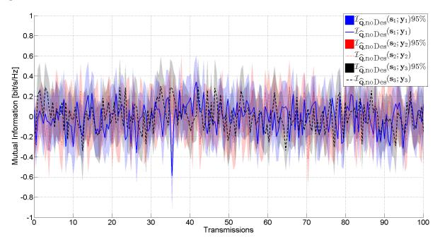
Figure 4.3.: Measurement of the MI where the desired transmitters were turned off, averaged over  $N_M = 50$  measurements with 95% confidence intervals of the mean
