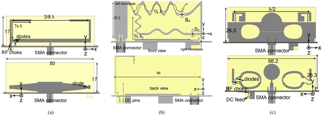
Fig. 2. Dimensions of the antenna prototypes. The antennas are denoted as a) antenna 1 (Reprinted with permission from [13]; ©2016 IEEE.), b) antenna 2 (Reprinted with permission from [14]; ©2016 IEEE.) and c) antenna 3 (Reprinted with permission from [15]; ©2017 IEEE.) Dimensions are in millimeter.
