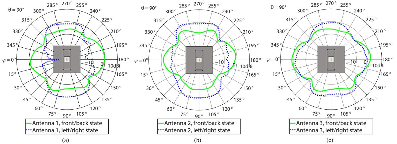
Fig. 5. Measured horizontal cuts of the gain patterns at 2.45 GHz for polar angle  $\theta = 90^\circ$  of a) antenna 1, b) antenna 2 and c) antenna 3. If the cavity is mounted on the vehicle according to Fig. 1, the left sides of the plots ( $\varphi = 0^\circ$ ) coincide with driving direction.
