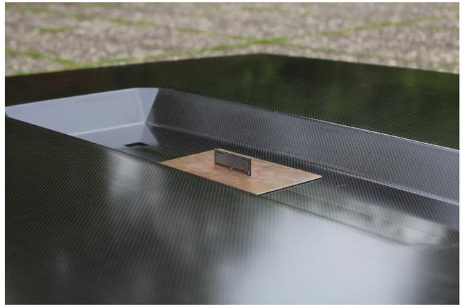
Fig. 3. Pattern reconfigurable antenna 1 inside the CFRP chassis antenna cavity.
