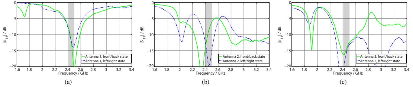
Fig. 4. Measured absolute values of the S-parameters with the antennas placed inside the chassis module a) antenna 1, b) antenna 2 and c) antenna 3.
