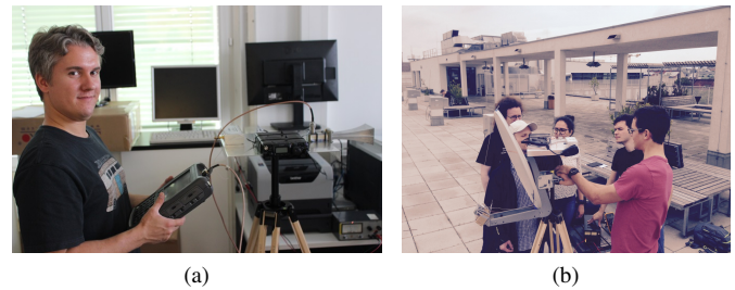
Fig. 2: The students are allowed to assemble transceiver configurations and enjoy the increased autonomy. a) Students have assembled a 3 cm setup with an amateur radio transceiver, a transverter and a horn antenna. A student tests the antenna with a handheld analyzer. b) Another group used a self-built horn antenna to feed an offset parabolic dish.
