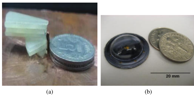
Fig. 9. a) Coins are used as a measurement unit in [34] in the sense that multiples of a base unit are used. Three coins are stacked to measure the height as 3 \cdot \text{thickness} (5 INR). Copyright © 2019, IEEE. b) Coins are used as a measurement unit in [35] in the sense that fractions of a base unit are used, image used with permission.
