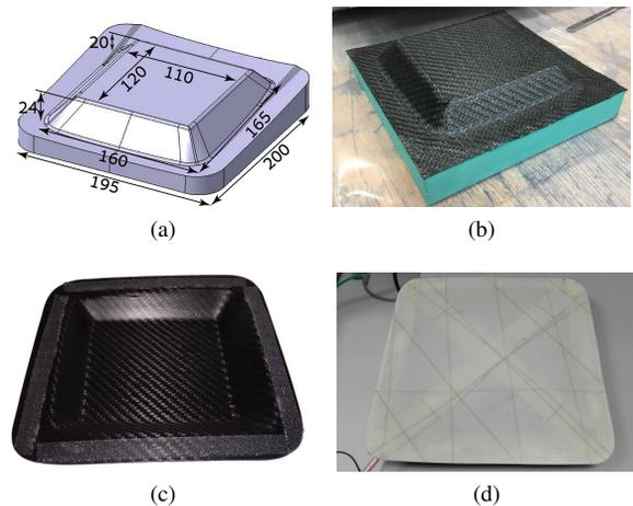
Fig. 2. The antenna cavity at various stages of production. a) CAD model of the mold, b) mold with prepreg before vacuum bagging, c) CFRP cavity and d) cavity with glass-fiber reinforced protective cover.
