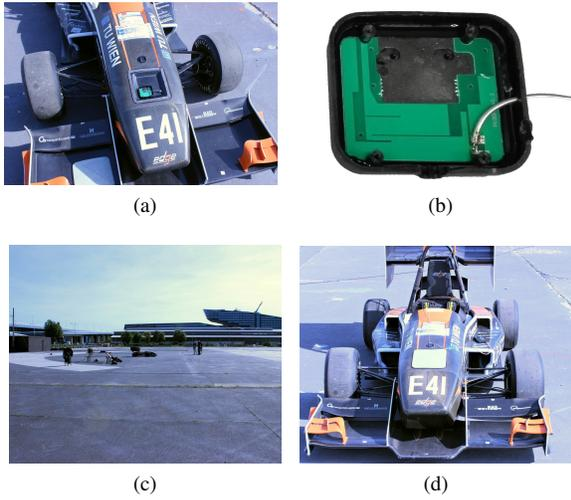
Fig. 3. a) EDGE 9 with the antenna cavity inserted into the monocoque. b) Off-the-shelf antenna that is used to evaluate the antenna cavity. c) Measurement of the radiation patterns on the outdoor range. d) Racing car with conformal antenna cavity.
