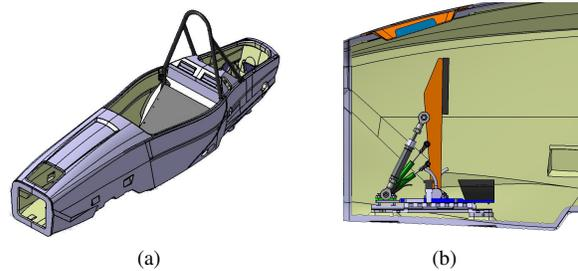
Fig. 1. a) CAD drawing of the racing car monocoque. b) Monocoque front part with the pedals and the antenna cavity above them.
