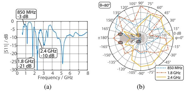
Fig. 4. a) Measured S-parameters of the off-the-shelf antenna inside the covered CFRP antenna cavity. b) Measured normalized radiation patterns;  $\theta = 80^\circ$ ; vertical polarization.
